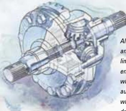
*All Outback models except Outback Sport and Outback H6-3.0 VDC feature a standard limited-slip rear differential that further enhances rear wheel traction. If one rear wheel starts to lose traction, power is automatically diverted to the other rear wheel—all without the need for driver intervention.*
